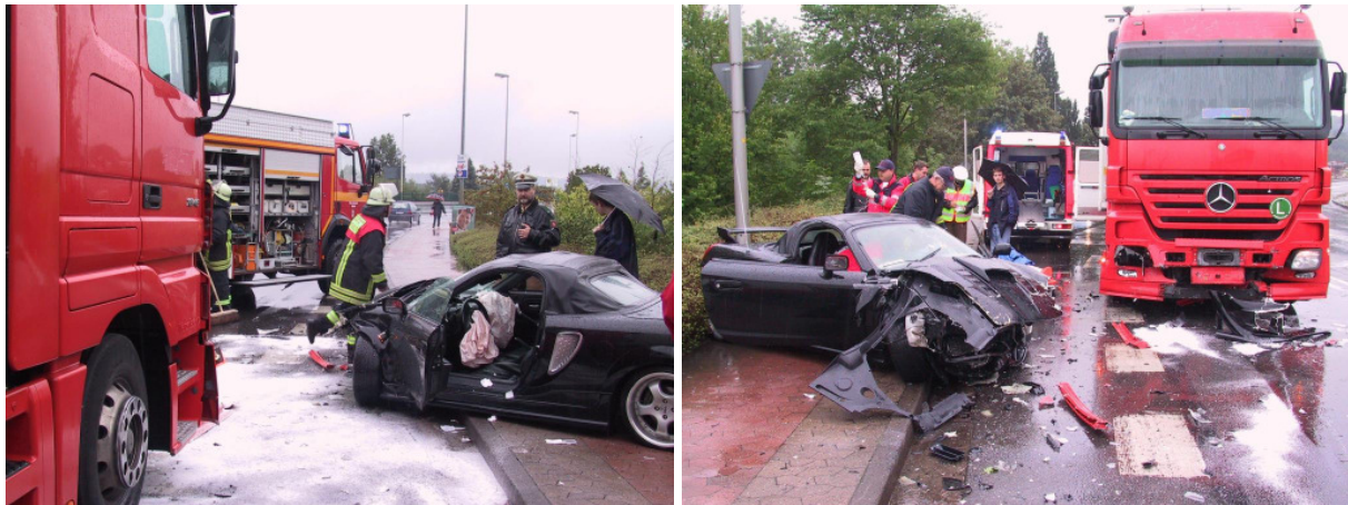
Fig. 6, 7: Frontal collision between passenger car and truck with front underrun protection (source: Kreispressewart Friedrich W. Thies, Hameln)
