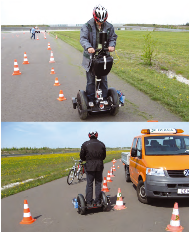
Picture 5: Driven sections of the test track (top: braking, bottom: obscured sight)
