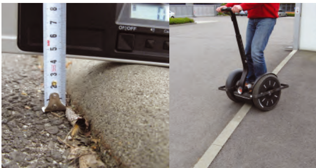
Picture 2: Unproblematical manoeuvring of a lowered kerbstone
