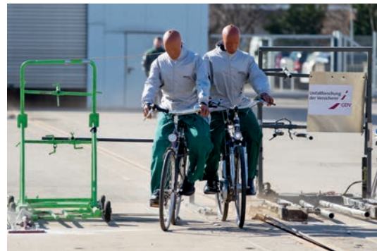
Figure 2: Collision between a bicycle (at 22 km/h) and an overtaking pedelec (at 44 km/h).
