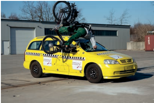
Figure 3: Collision between a stationary car and a pedelec coming from the side (at a speed of 44 km/h)
