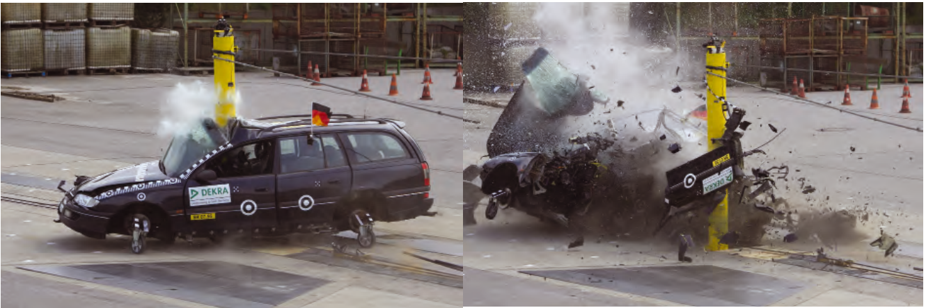
Figure 7: Collision of a 1994 Opel Omega B with a pole at 97 kph at an angle of 23° and with a test weight of 1,656 kg [5]
