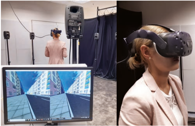
Left: Setup of the 16 speakers in the lab and visual presentation of the street scene with vehicle. Right: Test subject with VR goggles.
