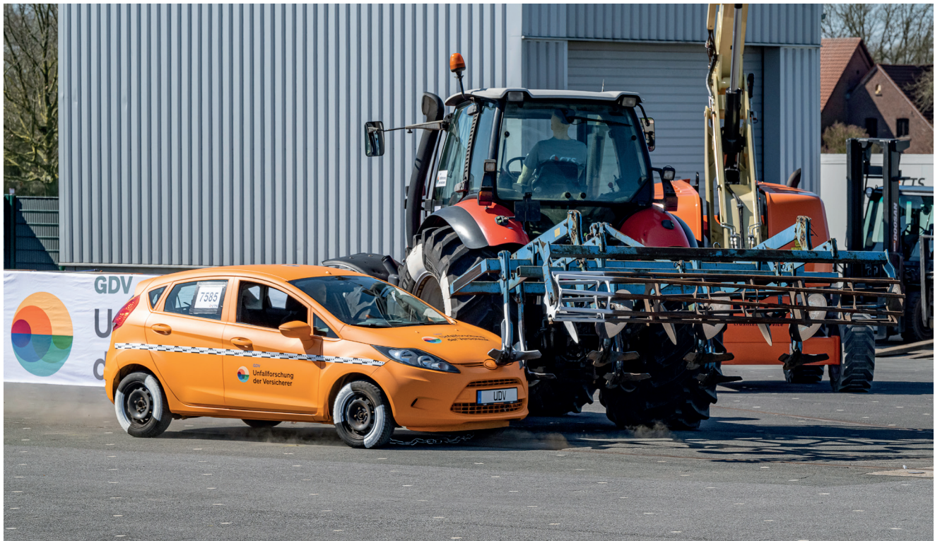
Figure 1 · Size comparison of cars and MAV and capacity to inflict damage due to the geometry of the attachments
