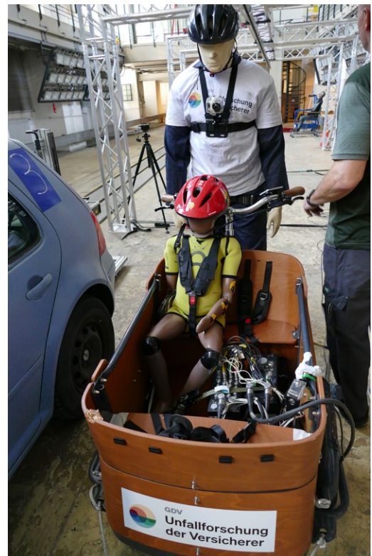
Figure 13 · Cargo bicycle with crash test dummies
