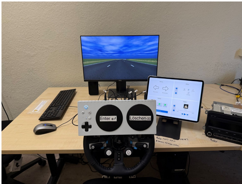
Figure 6: Basic driving simulator setup used for all three generic HMIs (physical controls, touch-based, speech-based).
