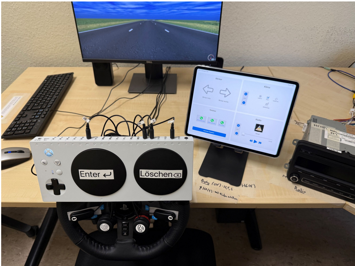
Experimental setup of the physically controlled HMI.
