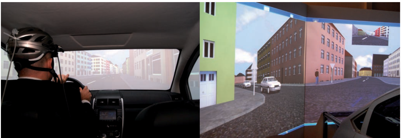
Figure 3: Driving Simulator environment with Subject and gaze measurement device (left) and a typical built-up scene (right)
