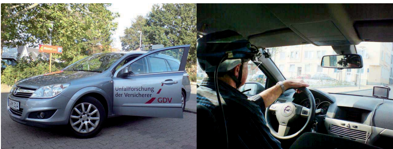
Figure 1: Experimental vehicle (left) and test person with gaze measurement device (right)
