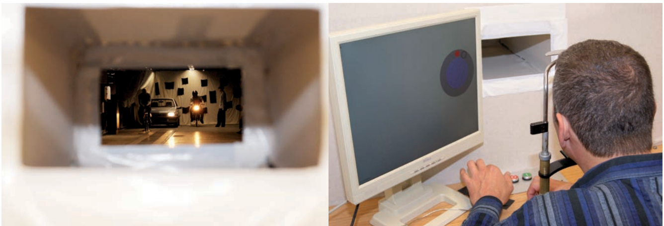
Figure 2: Test persons's view at the scene (left) and positioning of test person with tracking task (right)
