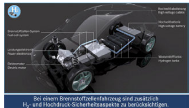
Figure 2: Parts of a fuel cell vehicle
