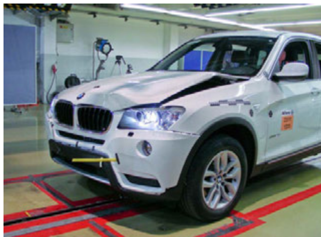
Figure 1: Typical scope of damage after an RCAR frontal crash at 15 km/h
