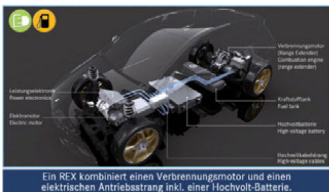
Figure 1: The range extender combines the advantages of both powertrain technologies
