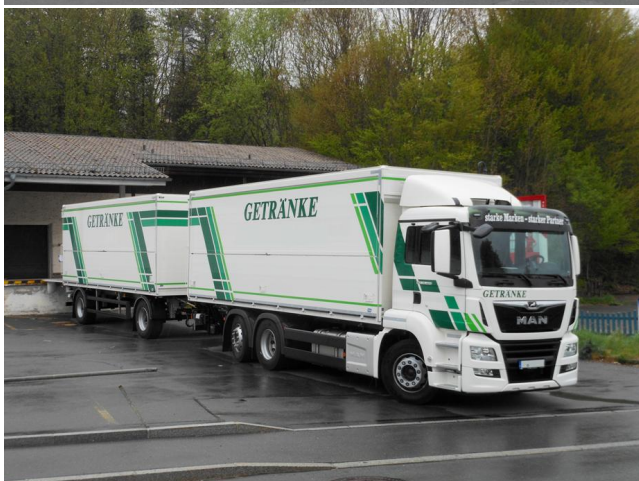
Fig. 1. Examples of rigid trucks (above left: 11,990 kg GVW, N2; above right: 32,000 kg GVW, N3), rigid truck (below left: 26,000 kg GVW, N3) with drawbar-trailer, and semi-tractor (below right: 18,000 kg GVW, N3) with semi-trailer.
